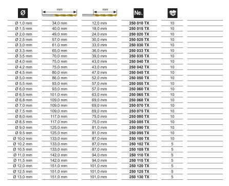
Twist drills DIN 338 type N HSS-TiN ground in plastic case
